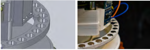
Figure 20: Hall effect sensor positioning relative to magnetic encoder ring.
