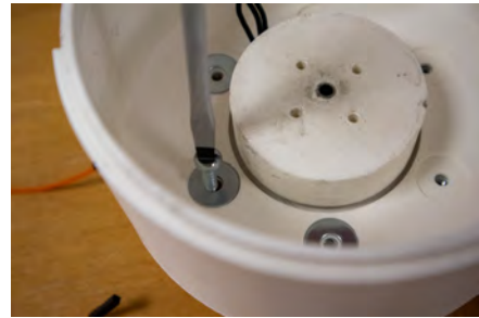
Figure 17: Recesses for washers
