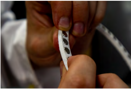
Figure 9: Magnets fitted to encoder ring
