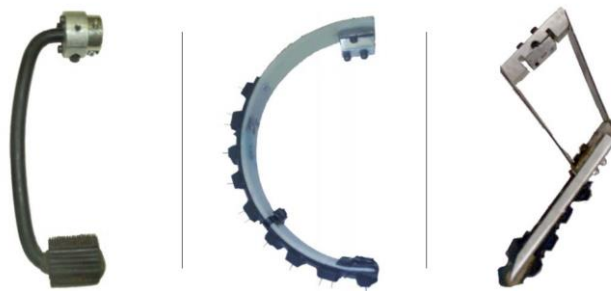
Figure 7 – Compass leg design (left), C-shaped leg design (middle), Hinged four-bar leg design (right)
