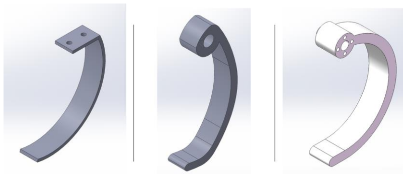
Figure 8 – Iterations 1, 2,3 for the Rhex's legs
