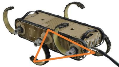
Figure 2 – Annotated diagram of RHex loaded legs create a triangle structure while moving (5)
