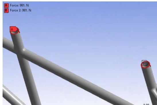
Figure 5: Weight of riders acting on seat posts
